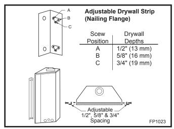
Fig. 4 Adjustable drywall strip (nailing flange).
